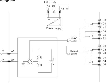
The battery connections are to be done at A3 and A4
