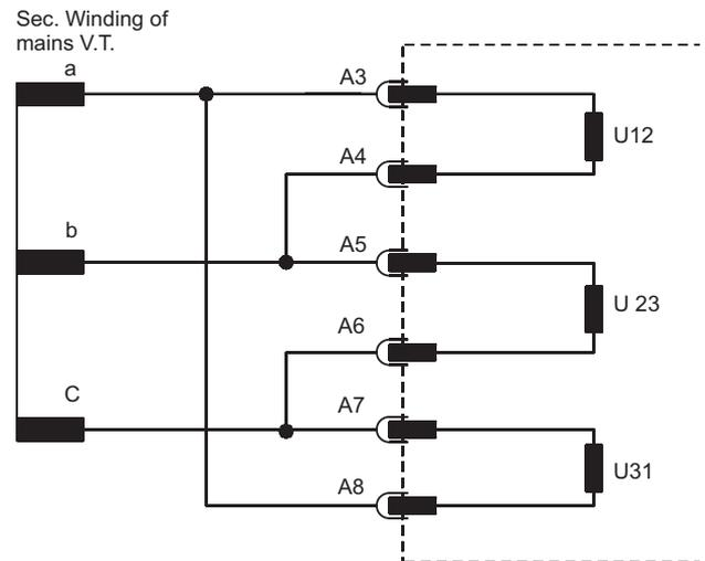
Fig. 4.1: Input v.t.s in delta connection ( $\Delta$ )
