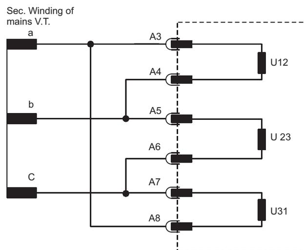
Fig. 4.1: Input v.t.s in delta connection ( $\Delta$ )
