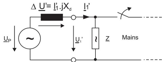
Fig. 4.6: Equivalent circuit at mains failure
