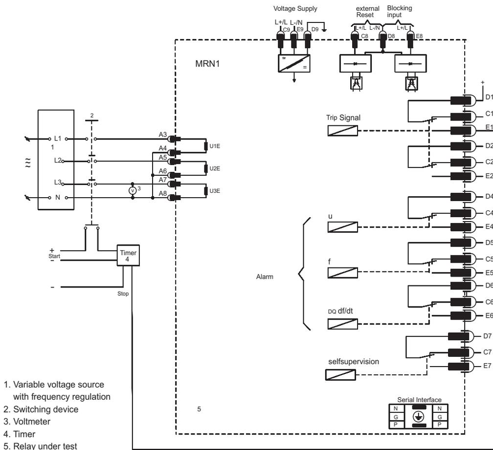
Fig. 6.1: Test circuit
