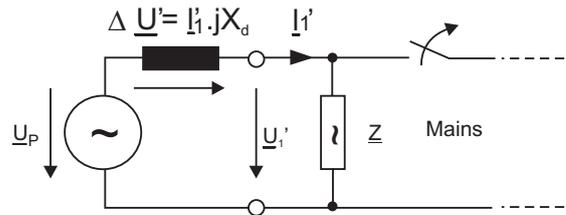
Fig. 4.6: Equivalent circuit at mains failure
