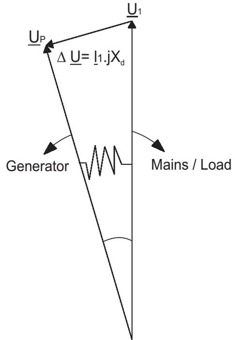
Fig. 4.5: Voltage vectors at mains parallel operation
