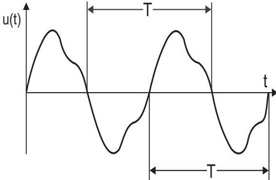
Fig. 4.3: Determination of cycle duration by means of zero passages.
