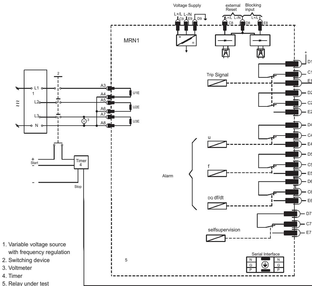
Fig. 6.1: Test circuit
