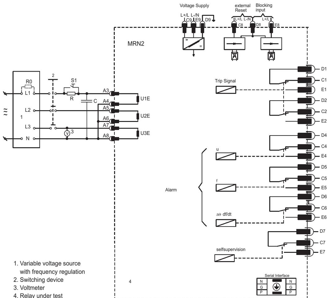
Fig. 6.2: Test circuit for the vector surge function
