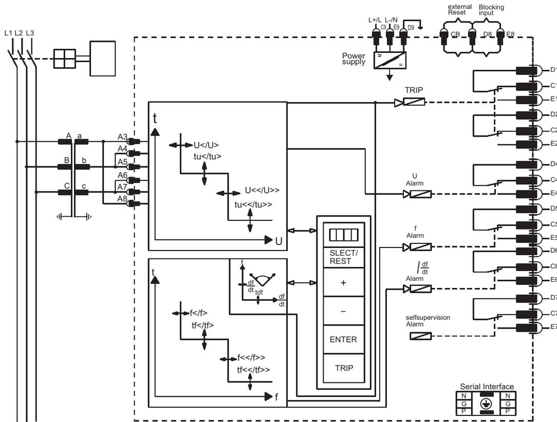
Fig. 3.1 : Connection diagram MRN2-1 and MRN2-2
