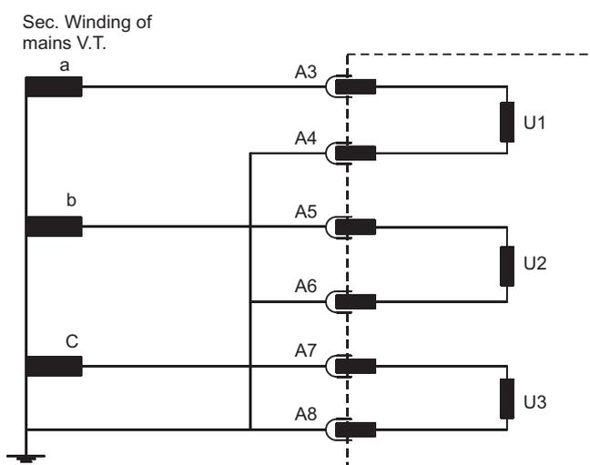
Fig. 4.2: Input v.t.s in star connection (Y)
