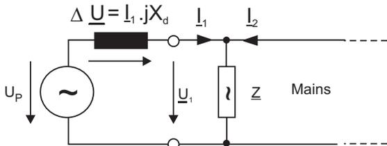
Fig. 4.4: Equivalent circuit at synchronous generator in parallel with the mains
