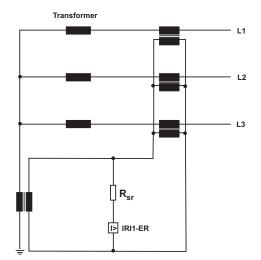
Fig. 2.1: Zero-current differential protection of a transformer in star-connection (IRI1-ER)
