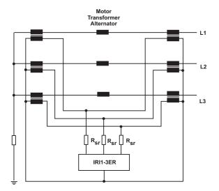
Fig. 2.2: Highly stabilized differential protection for alternators, transformers and motors (IRI-3ER)
